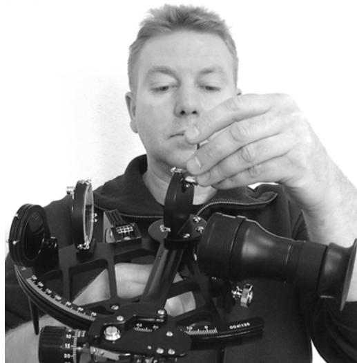
Take the sextant this way to identify and correct tilt error of index mirror.
